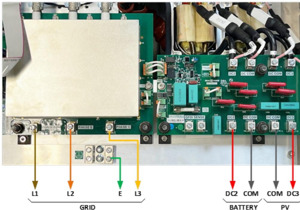
Figure 3: AC1, DC2 and DC3 power connection terminals
