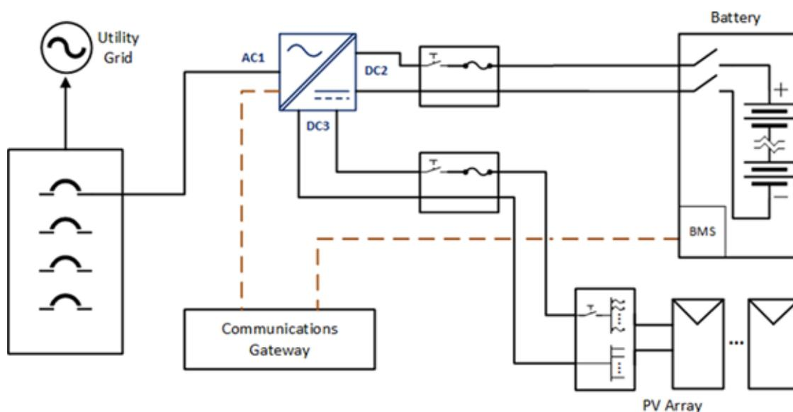
Figure 5: Typical PCS battery and PV system connections
